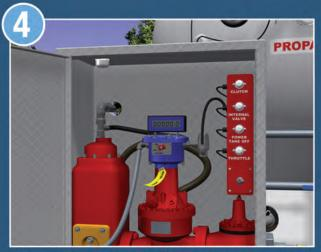
Engage the Power Take-Off (PTO) to start the pump. NOTE: To prevent pump damage, do not increase the engine speed above idle.
