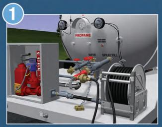
Connect the delivery hose-end valve adapter to the cargo tank liquid fill connection (using a male-to-female ACME adapter) or to the vapor equalizing connection.
