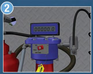
Start the vehicle engine and run it at idle. Prepare the truck meter according to your company's operating procedures and/or the truck manufacturer's instructions.
