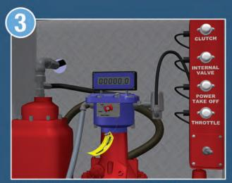
Open all necessary valves, including the liquid internal valve, the differential bypass valve, and other shutoff valves that may be in the piping system.
