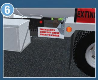
After establishing product flow, close the liquid internal valve using the emergency discharge control equipment on the truck. NOTE: Do not use the off-truck remote control devince during this test because it could shut off the truck engine.
