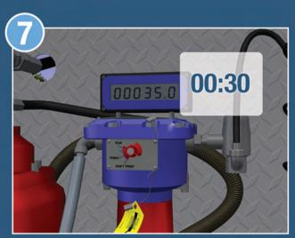
Carefully observe the truck's meter. All product flow must stop within 30 seconds. Continue the test for a maximum of 5 seconds after the meter stops. Any detectable meter creep within five seconds indicates the liquid internal valve is not fully closing and is cause to remove the vehicle from service until repairs or replacements are made.
